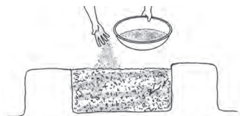
Fig. 57. Adding ash to the second pit
